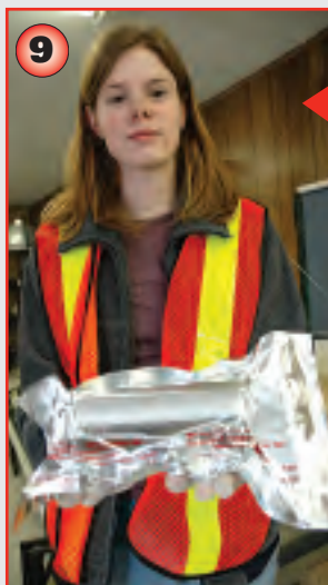
9. The core sample is then placed in a foil bag for added protection and sent off for testing. Some samples will be maintained in a refrigerator to recreate insitu temperatures between four and 10 degrees. On site testing of core samples for strength and the ability to withstand weathering as well as other geomechanical field tests will take place while many of the roughly 300 core samples expected to come from each borehole will be sent to laboratories across the province including those at the University of Ottawa. Some cores samples will also be sent to the University of Bern in Switzerland for chemical analysis of pore water.
