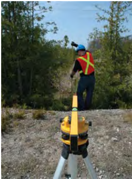
AMEC engineer Peter Nimmrichter measures the elevation change across a culvert at the Bruce nuclear site as part of the mapping of the site drainage network. The information will be used in the safety assessment currently being compiled by NWMO on behalf of OPG.
