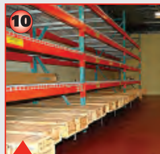
10. Every piece of core is carefully logged and accounted for and all lengths must be stored in wooden boxes in the core storage facility with proper identification. Wooden plugs will be used to fill the holes left by the removal of core samples.
