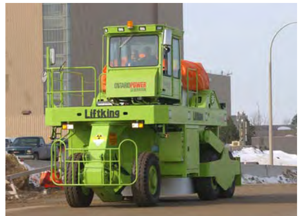
OPG staff safely transporting the first Dry Storage Container (DSC) from Bruce B over to the Western Used Fuel Dry Storage Facility (WUFDSE).
