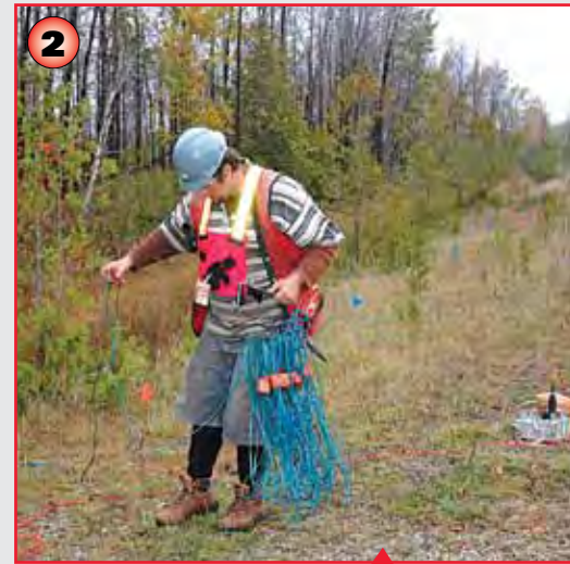
2. Geophones and seismic cables are placed along designated seismic lines.
