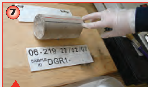
7. Note the red (right) and black (left) lines drawn on the core sample to ensure that its orientation underground is known.
