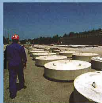
Intermediate level waste inserted into in-ground storage containers at the WWMF
