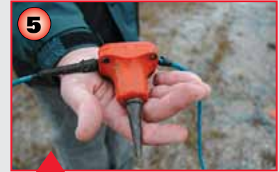
5. Geophones measure the magnitude and travel time of the vibrations from underneath the surface.
