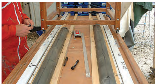
Core samples are recovered and logged during the drilling process. They will be carefully stored according to established specific quality assurance methods that will safeguard the integrity of all data and samples generated as a result of site characterization activities.
