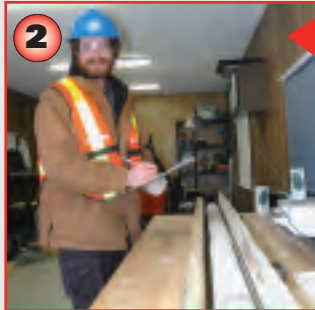
3. Core is only handled using gloves to maintain its integrity and prevent contamination from outside sources.
