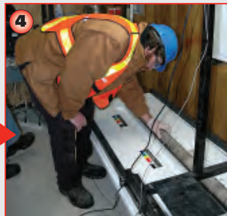
2. Core from the drill site is received inside a dual tube system core barrel which allows the core to be pulled out in three metre lengths without taking out the drill rods. Once the core comes up, it is immediately taken to the core receiving trailer set up on site. Glen Briscoe, site supervisor from Intera Engineering - the Ottawa company charged with preparing and overseeing the geoscientific site characterization program for the proposed DGR - shows how the core, in a split core barrel, is laid out in the DGR CORE SLED for photography and logging.
