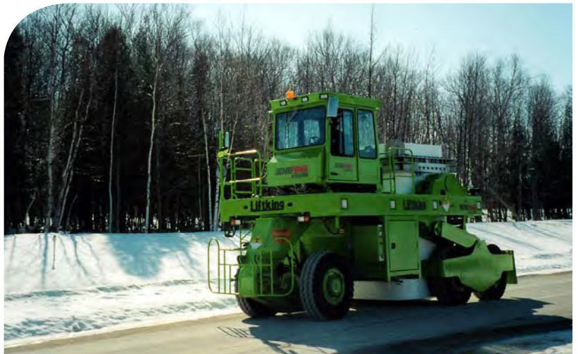
WWMF staff transporting a Dry Storage Container on site from Bruce Power's Bruce B station to the Western Used Fuel Dry Storage Facility
