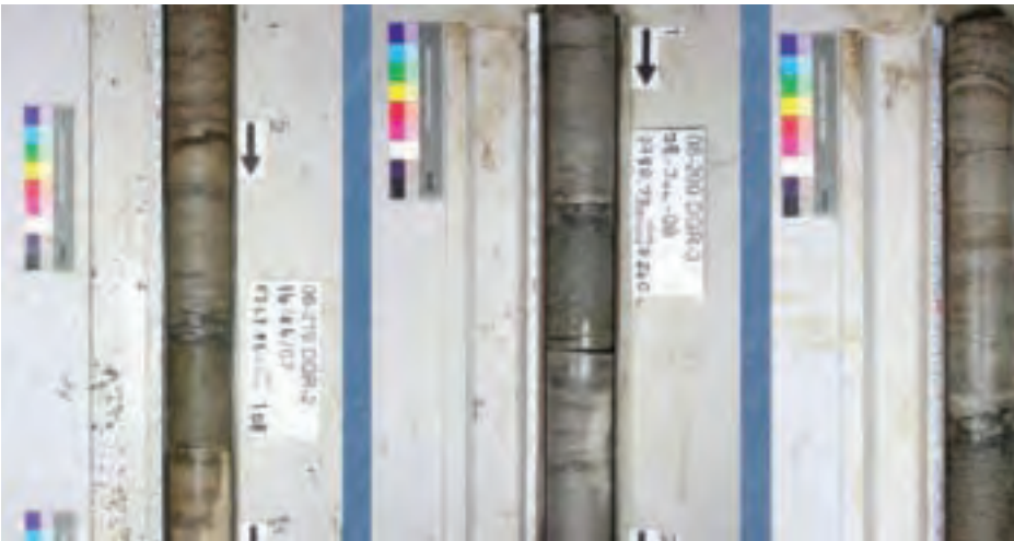
The layer of Bentonite found in core samples from three different boreholes speaks to the consistency of the geologic layers.
