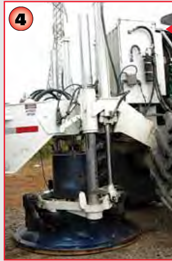
4. A hydraulically activated pad on the vibroseis truck is utilized to send vibrations that travel through the subsurface down to the Precambrian basement and back up to the surface.
