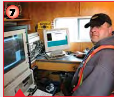
7. Data from geophones is transferred to a collection box and then on to the recorder truck where it becomes part of a seismograph.
