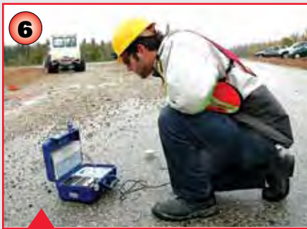
6. The vibrations created by the vibroseis truck are measured and monitored with a ground motion measuring instrument to ensure they are within an acceptable range.
